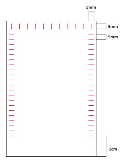
Once it's all marked off, carefully use the chisel and mallet to punch holes where the marks are. Try and make sure the holes down the length of the leather line up.
