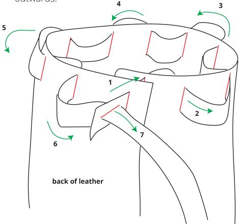
Use the thong to stitch the leather through holes as shown in the diagram (the pliars help) starting with position #1 (the end with the hole cut in the thong). NOTE: the first stitch goes through two holes. When you go through the last hole, put the thong through itself.
