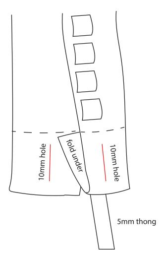
Using the 10mm chisel, punch 2 holes through the folded area at the bottom of the leather, making sure to go through both layers. Additionally the holes should run parallel with the length of the bag.
